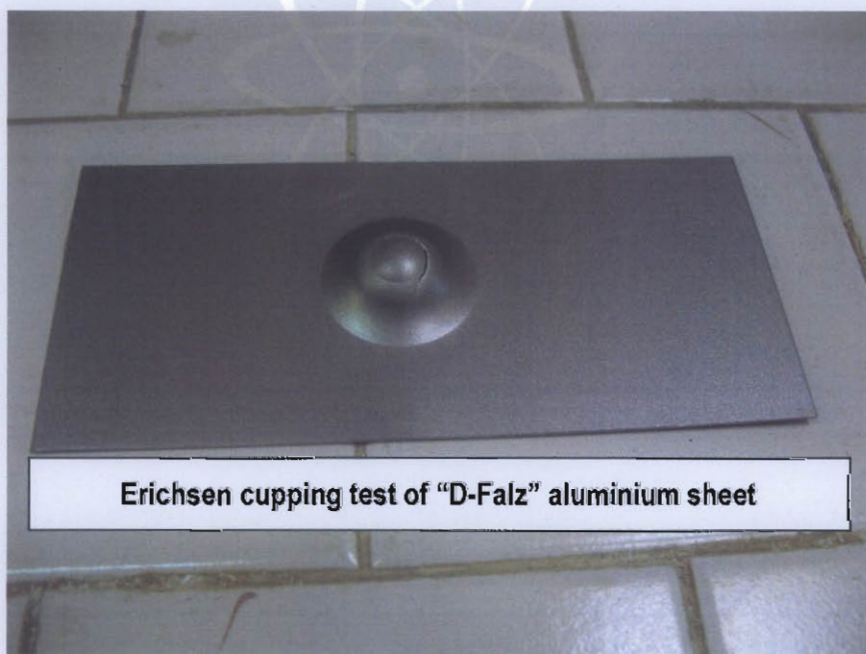
Photo of sample after Erichsen cupping test.
